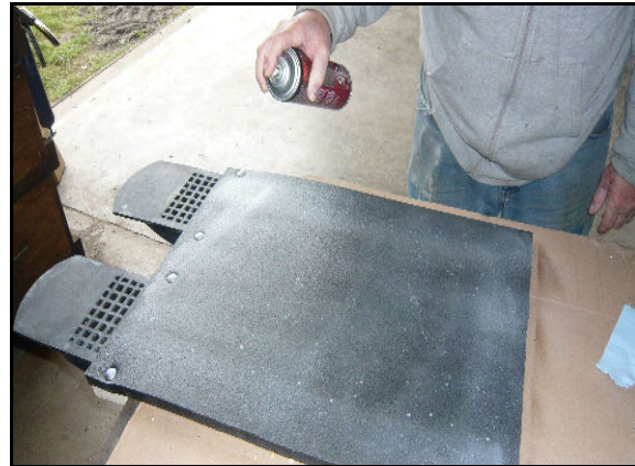
FIG. 1-7. Applying the Adhesive
