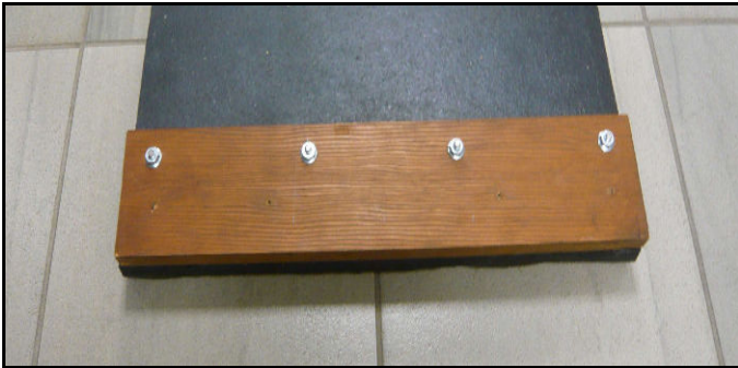
FIG. 1-5. Installing the Spacer
